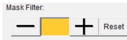
To add blocks, click + button; to erase blocks, click - button. Click 'Reset' button to reset motion detection blocks to default setting. You can also change the color of block if its color is similar to the IP camera's video and makes you hard to identify the blocks by click the color brick between + and - button:
